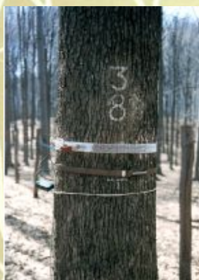
Automatic (above) and manual (below) girth band
