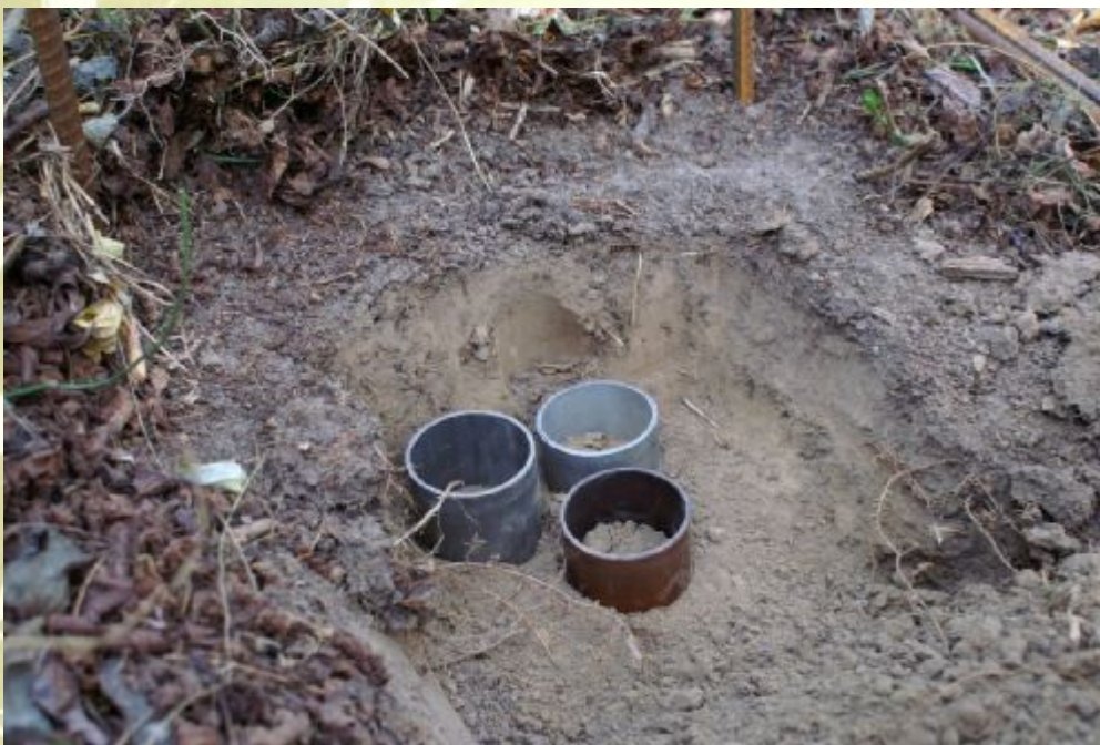
Cylinders with a volume of 100 cm 3
